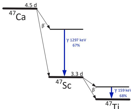
**Figure 2:** A simplified decay scheme for  $^{47}\text{Ca}$  and  $^{47}\text{Sc}$ . The low energy beta particles from  $^{47}\text{Sc}$  are therapeutic, and the 159 keV gamma ray has an appropriate energy for imaging with single photon computed tomography (SPECT).
