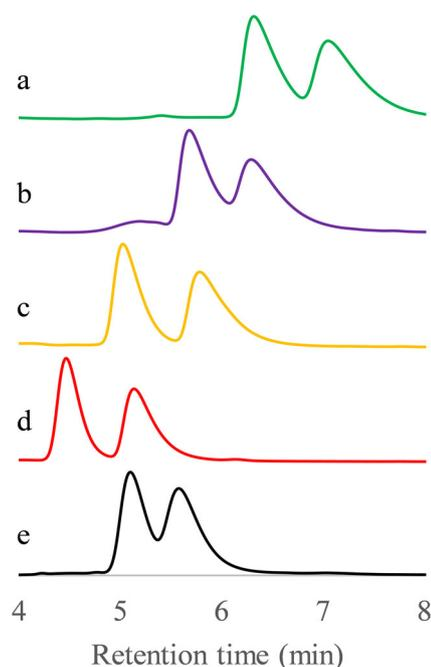
**Fig. 6** Retention times for *cis* and *trans* DDSQ-(Ph)<sub>8</sub>(hydroxyl)(R<sup>2</sup>). (a) R<sup>2</sup>: methyl 6; (b) R<sup>2</sup>: vinyl 7; (c) R<sup>2</sup>: isopropyl 8; (d) R<sup>2</sup>: isobutyl 9; and (e) R<sup>2</sup>: phenyl 10
