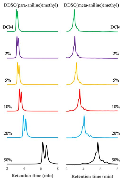
**Fig. 4** Effect of dichloromethane/hexane mobile phase ratios in normal phase pHPLC for *cis-trans* of **2** and **3**. The percentage value indicated represents the volume percentage of hexanes in the mobile phase
