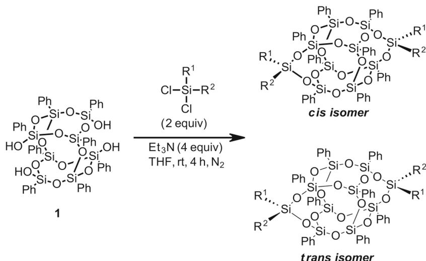
hydrolysis reaction producing a mixture of DDSQ cages including *cis* and *trans* isomers functionalized with hydroxyl groups. It was found that *cis* and *trans* isomers may be separated by a preparatory silica column and fractions quantified by HPLC [8, 12, 15].
