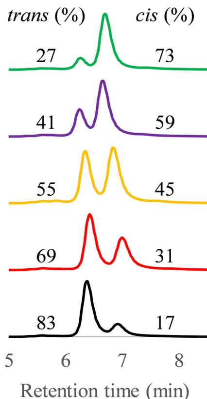
**Fig. 5** Quantitative analysis of *cis-trans* mixtures of DDSQ-(Ph)<sub>8</sub>(*p*-aniline)(methyl) by pHPLC. The individual isomers were first isolated and then mixed to a known ratio for comparison against the area under each peak. The weighted percent of isolated isomers in mixtures was indicated next to each curve
